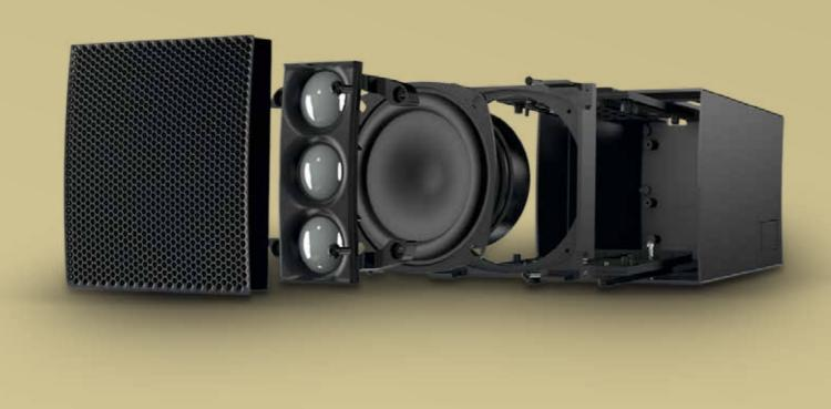
LD Systems' WaveAhead® technology places a vertical tweeter array in front of a high-performance full range transducer. This proprietary design reduces reflections from ceilings and floors resulting in clear, consistent coverage.
