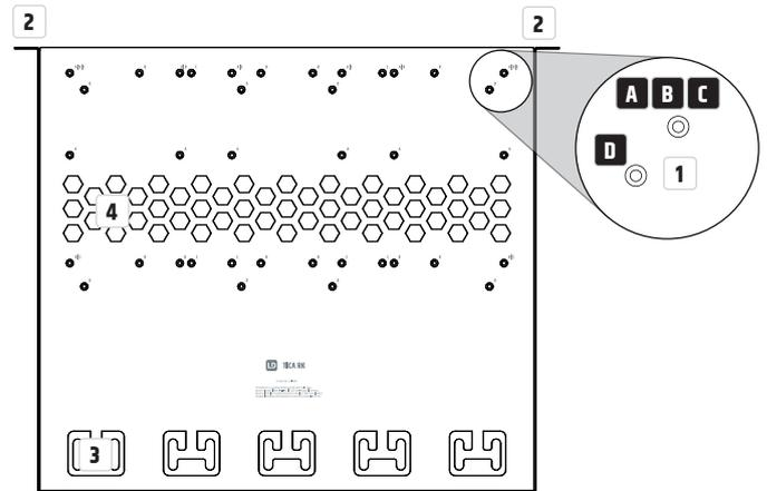
Front plates in various widths are included in the packaging content. The corresponding front plate is screwed tightly into a gap between two units on the rack tray to get a closed front
