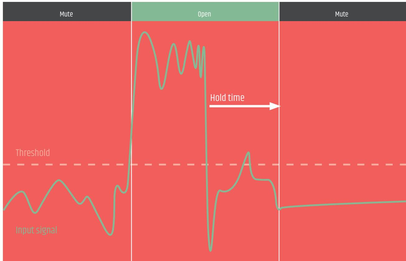
The U500 receiver's noise gate provides a choice of AUTOMATIC or MANUAL modes of threshold and hold time setting.
